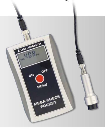
With the LIST MAGNETIK MEGA-CHECK Pocket coating thickness meters, you can carry out exact, reproducible measurements. The measuring probes digitize the signals in the probe before they are transmitted to the measuring device via the probe cable. The probe cable, which can be plugged in on both sides, connects the display unit and probe, and can be easily replaced in the event of a cable defect.
