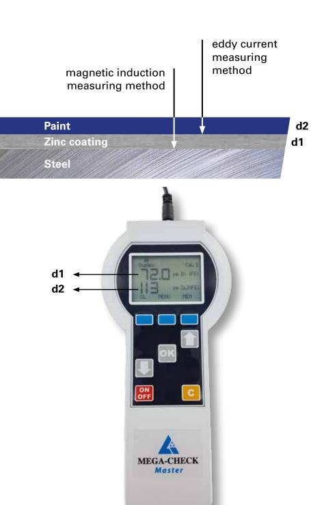
Two measuring techniques are used to measure the thickness of layers over a metal substrate.
